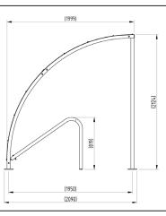
The VS1 Cycle Shelter is a light weight, free-standing, single sided cycle shelter with integrated cycle stands designed for on site assembly. Constructed from galvanised steel tube with a clear 4mm PET roof, the VS1 is supplied with integral bicycle stands for cycle storage.
