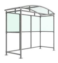
The Inglewood shelter is a free-standing, open fronted shelter designed for on site assembly, constructed from galvanised mild steel. Complete with a 4mm UV stabilised PETG clear sheet roof, and ½ side panels. Side-to side curved roof.
